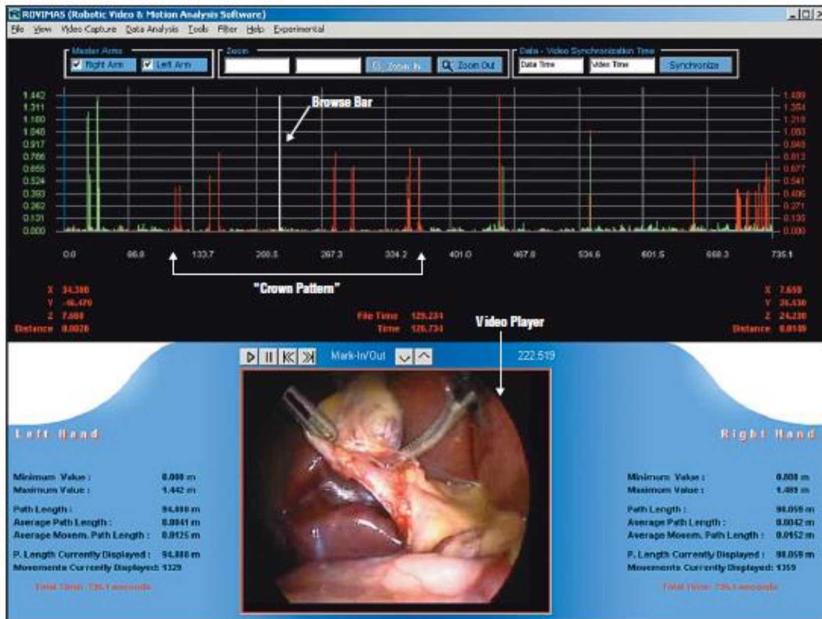
Figure 3. Snapshot of the Robotic Video and Motion Analysis Software (ROVIMAS) showing the crown pattern during a laparoscopic cholecystectomy case in which each pair of 2 high-velocity peaks represents extraction-insertion of the scissors-stapler instrument. Users can browse these data using the "browsing bar" and watch the corresponding video frames from the video player. P indicates path.
